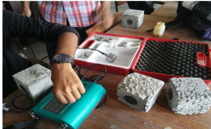
Fig. 5. UPV testing specimen
