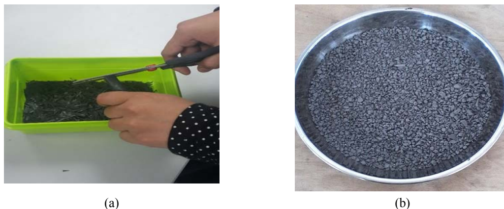
Fig. 4. (a) Manual extracting of waste plastic bag, (b) Crushed feedstock
