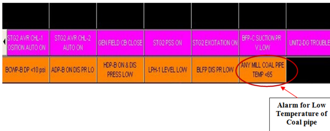
Fig. 6. Alarm Configured on Annunciation Panel.
