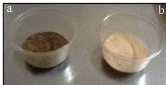
Fig.2. Treated fibers; (a) date palm leaves and (b) wood flour after sieving.
