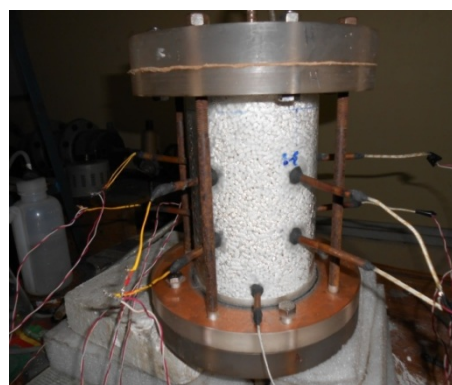
Fig. 3 Biogas passed through the scrubber
