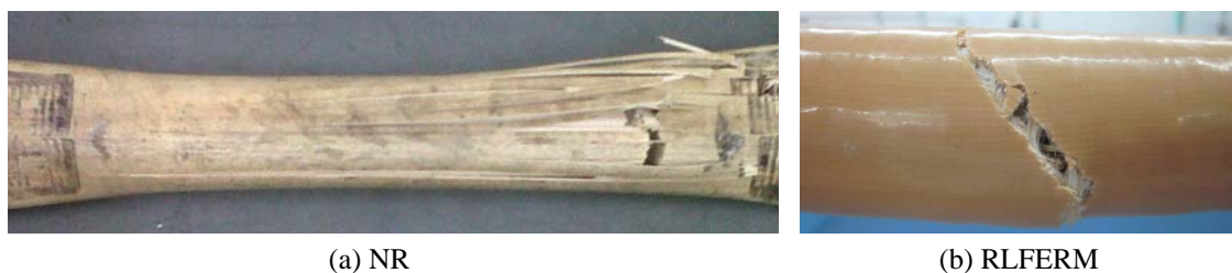
Fig. 4. Tensile Strength Sample Test of NR and RLFERM
