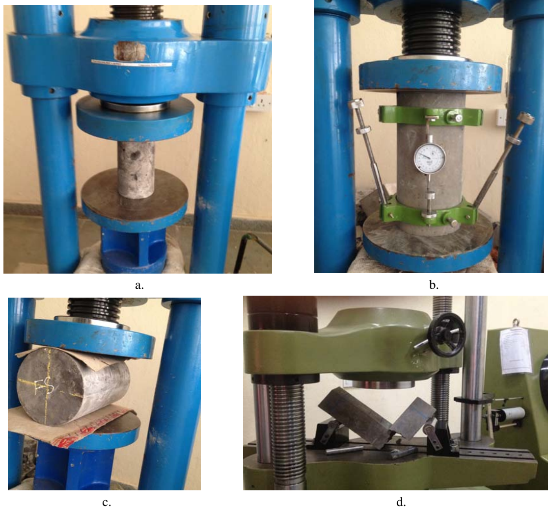
Fig. 4. Experimental test setup a) Compressive strength b) Modulus of elasticity c) Splitting tensile strength d) Flexural strength
