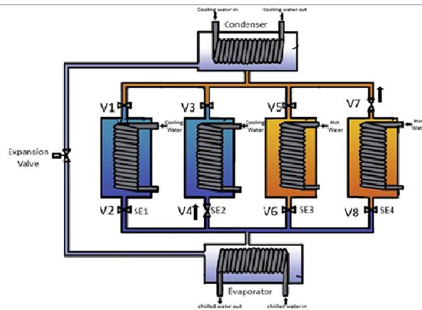
Fig.1: Schematic diagram of single stage four bed adsorption chiller
