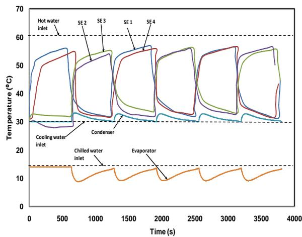
Fig. 4. Temperature profile of different components of two stage four bed adsorption chiller
