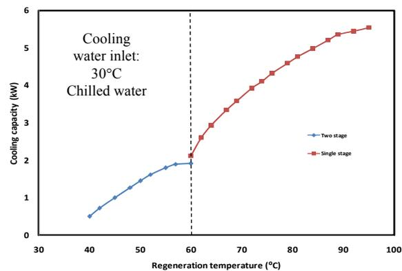
Fig. 5. Effects of cooling capacity on heat source temperature
