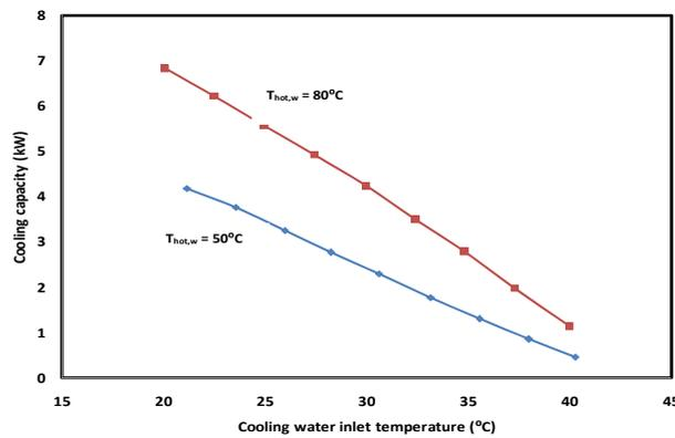
Fig.7. Effects of cooling capacity on cooling water inlet temperature
