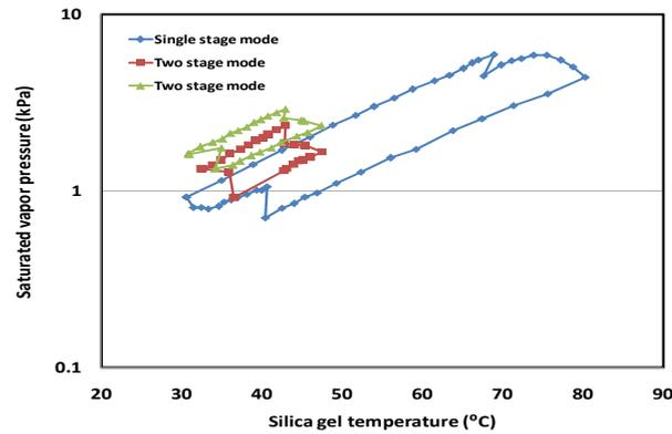
Fig.9. Dühring diagram of the dual mode adsorption chiller
