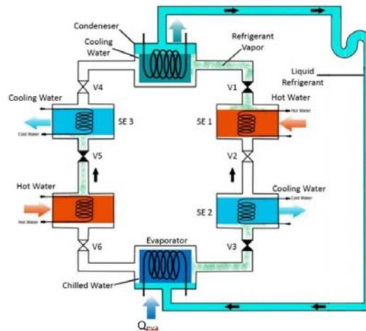
Fig. 2: Schematic diagram of two stage four bed adsorption chiller
