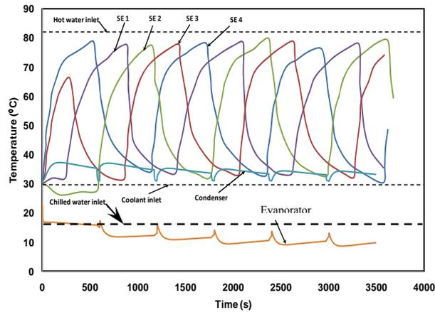
Fig. 3. Temperature profile of different components of single stage four bed adsorption chiller.
