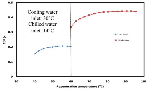
Fig. 6. Effects of COP on heat source temperature
