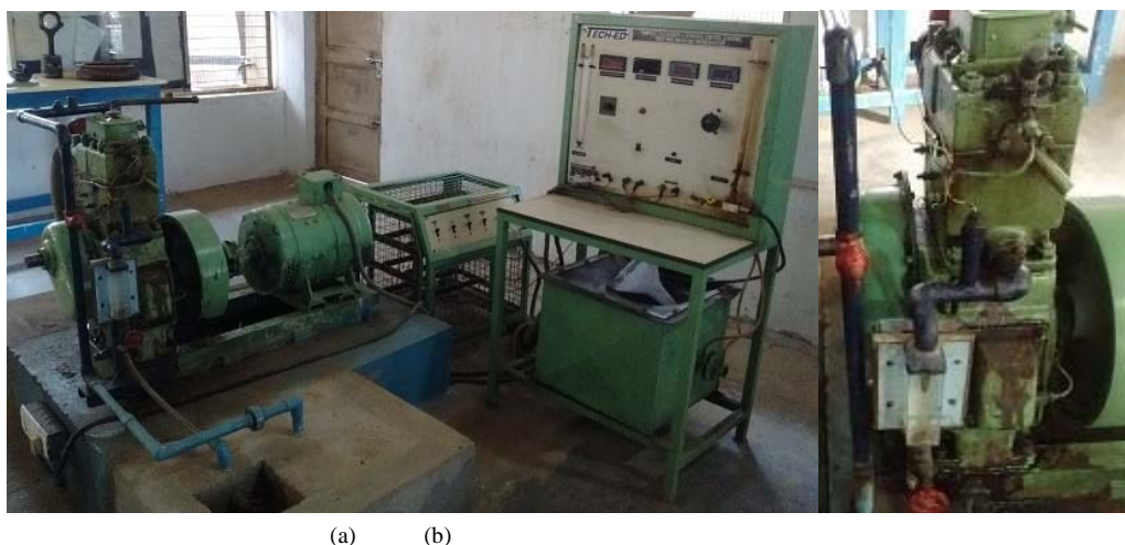
Fig. 3.(a) Experimental setup, (b) Engine with fuel injector operating at 200, 220 and 240 bar
