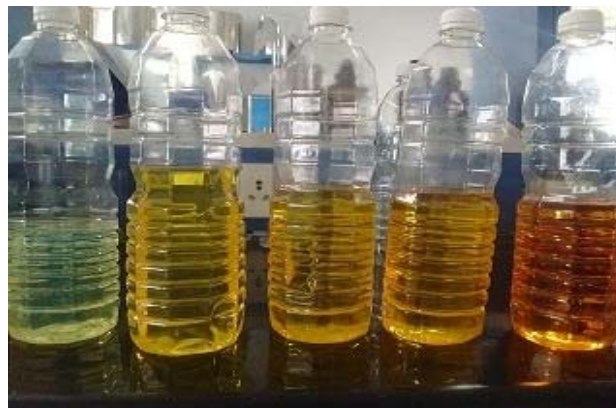
Fig. 2. Inside picture biodiesel-diesel blends (L10, L20 and L30) shown in the middle, mineral diesel and pure biodiesel are shown at the ends
