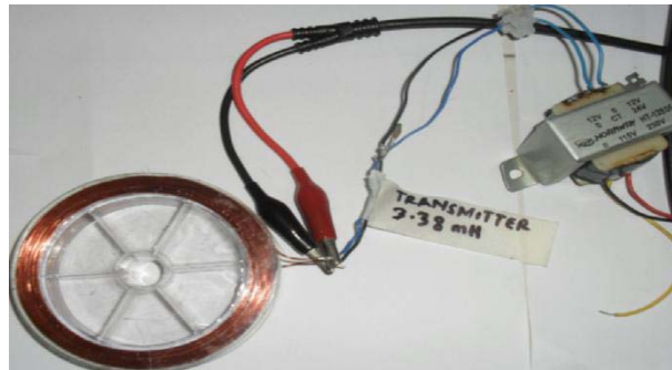
Fig 3. Coil connected in parallel with capacitor and in series with 12V step down transformer
