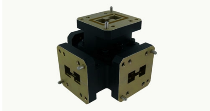
Fig.1. Schematic diagrams of 4 ports of double ridge waveguide coupler.
