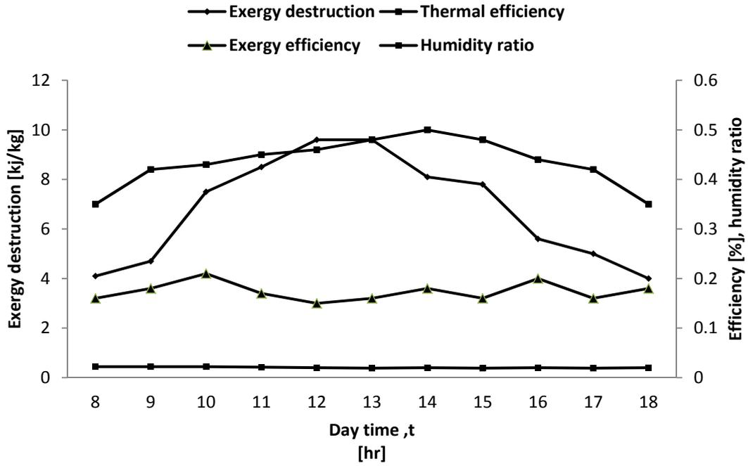
Figure 2 Curves of Efficiency, Exergy Destruction and Humidity Ratio in AH
