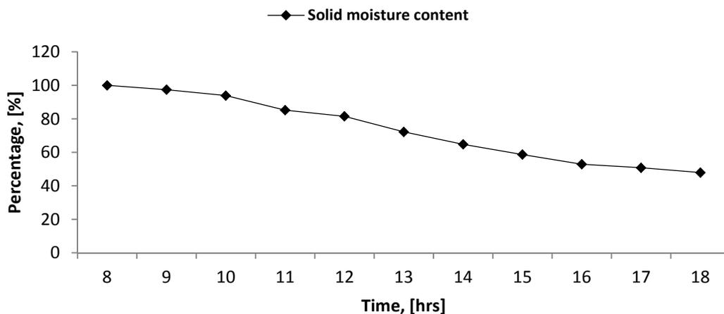
Figure 5 Curve of overall solid moisture content in MSD
