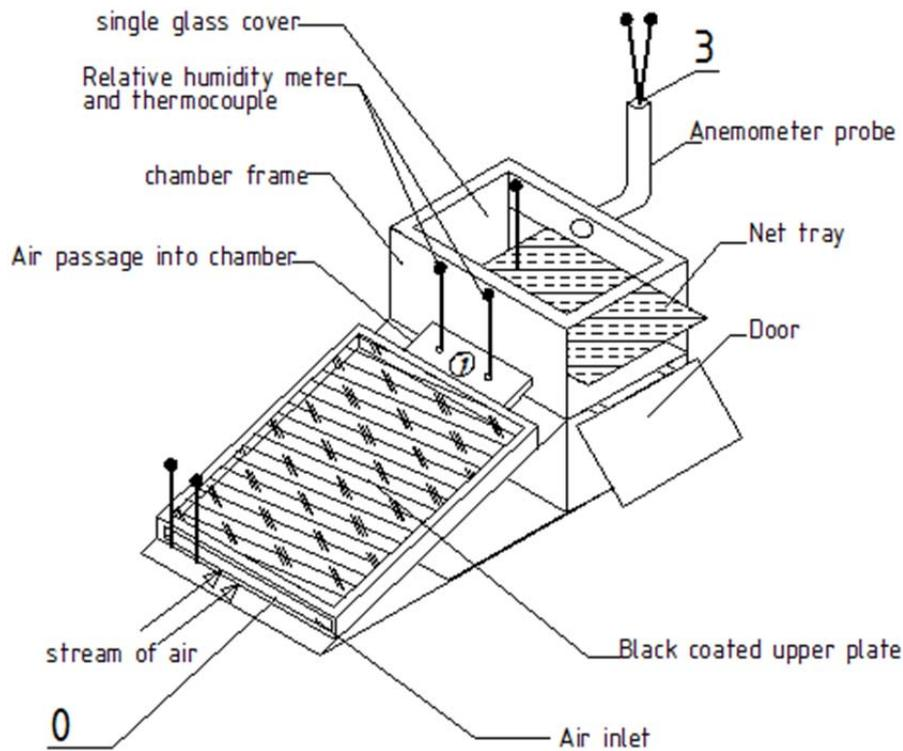
Figure 1(a) Schematic of Mixed-Mode Solar (MSD) Dryer
