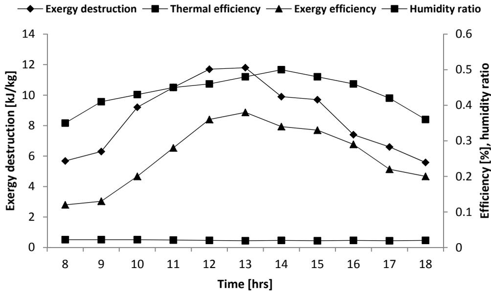
Figure 4 Curves of Overall Efficiency, Exergy Destruction and Humidity Ratio in MSD
