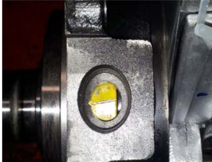
Fig. 10 Wrong Injection Timing
