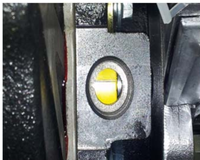
Fig: 13 Parallax Errors in FIP
