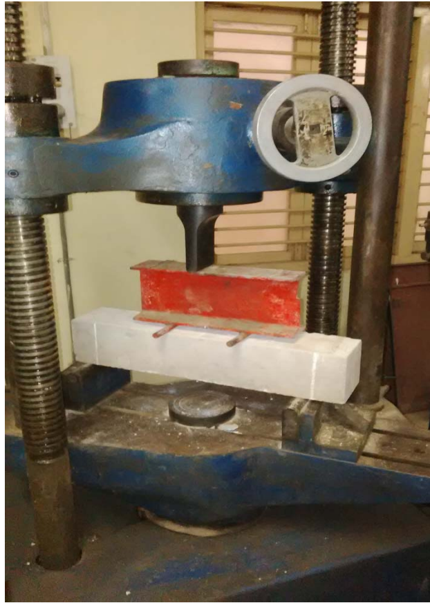
Fig. 2. Flexural strength test setup
