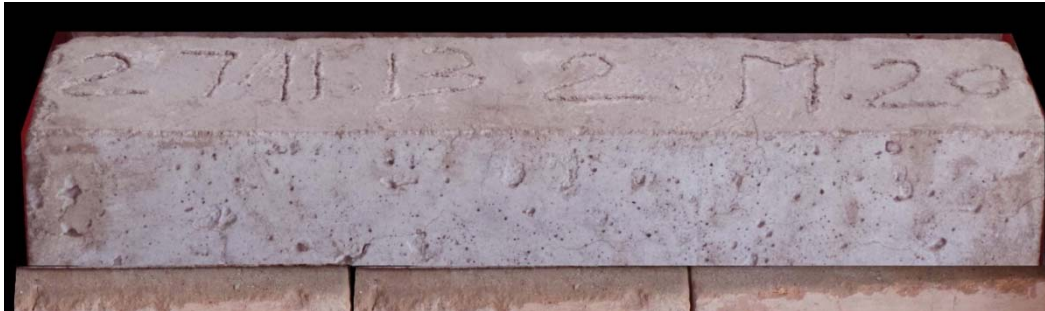
Fig.4(a). Crack pattern of GA concrete between 600 to 800 oC
