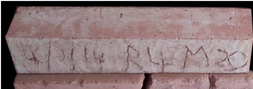
Fig.4(b). Crack pattern of RBA concrete between 600 to 800 oC
