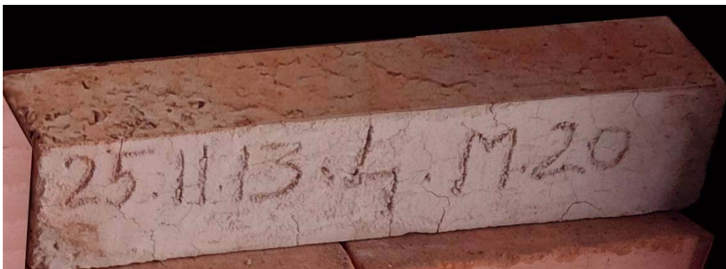
Fig.5(a). Crack pattern of GA concrete beyond 800 oC
