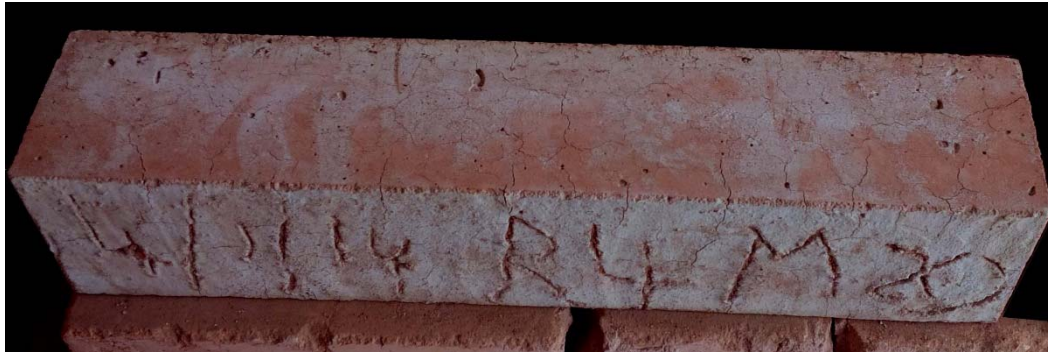
Fig.5(b). Crack pattern of RBA concrete beyond 800 oC
