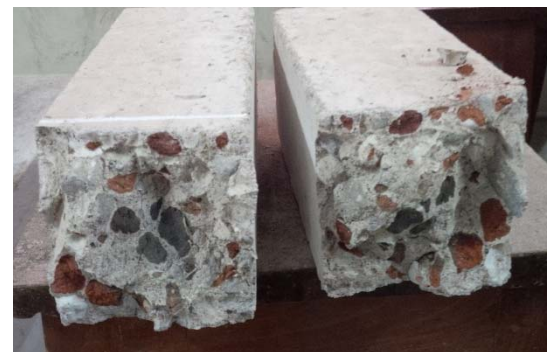
Fig. 7. Failure mode of RBA concrete
