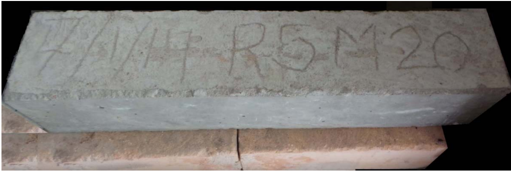
Fig.3(b). Crack pattern of RBA concrete upto 500 oC
