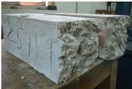
Fig. 6. Failure mode of GA concrete
