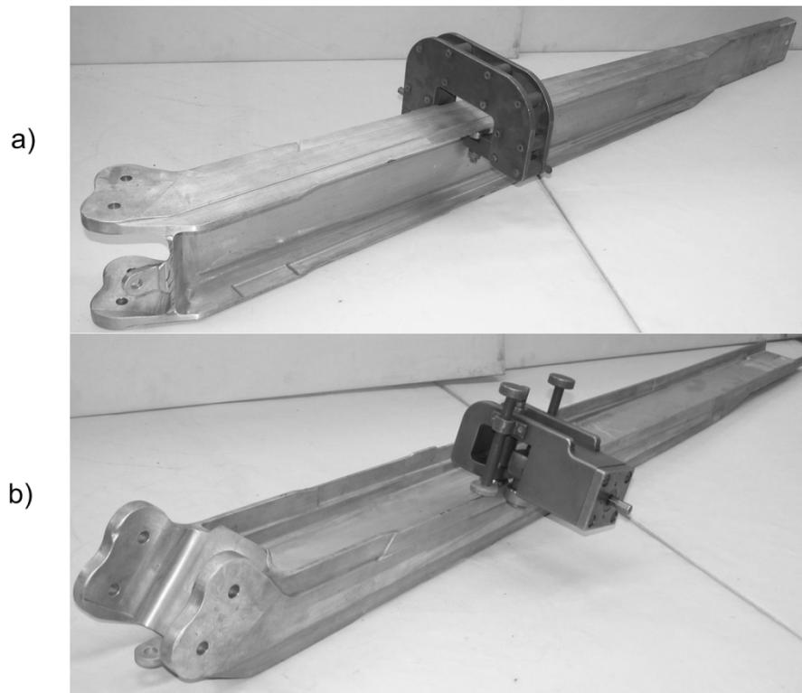
Figure 11 Tools for edge rolling (a) and sheet rolling (b)
