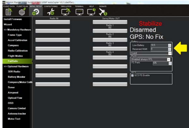
Fig. 3. Failsafe settings in Mission Planner
