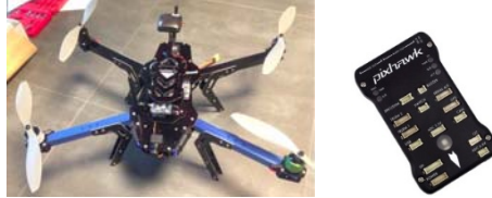
Fig. 1. 3DRobotics quadcopter and its Pixhawk used in the experiment
