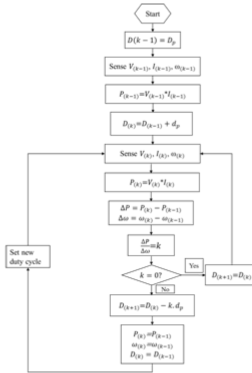
Fig.6 Proposed new, adaptive MPPT algorithm
