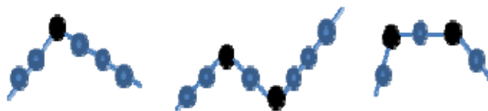
(a) peak (b) peak and valley (c) Clipping by Overloaded Figure 4 typical peak and valley and clipping by overload
