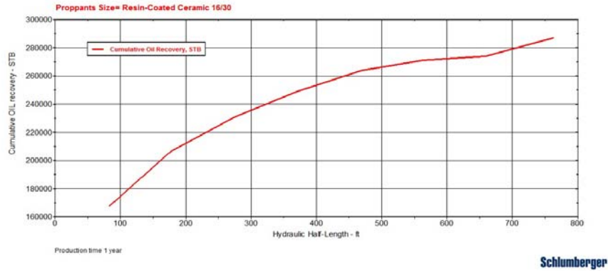
Fig. 22. Cumulative oil recovery versus fracture half length for proppant size equal to resin-coated ceramic 16/30
