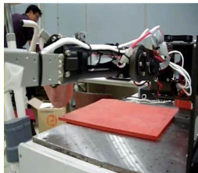
Fig. 10 Impact Test with Safe arm having variable stiffness joint
