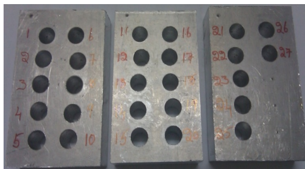
Fig. 3. Drilled Al7075-10%SiC p pieces
