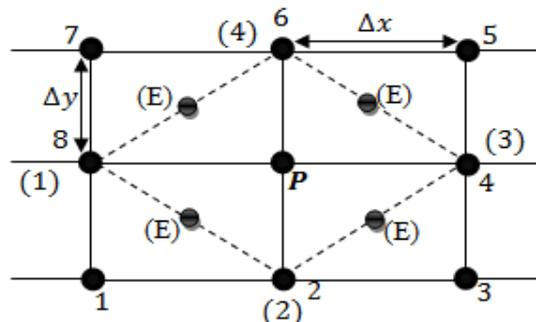
Fig. 2.The computational control volume structure.
