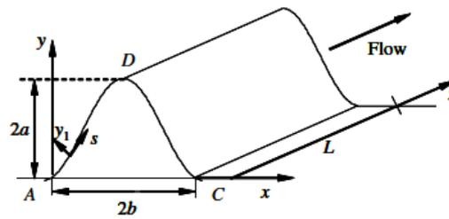
Fig. 1. Geometries of a sinusoidal duct.
