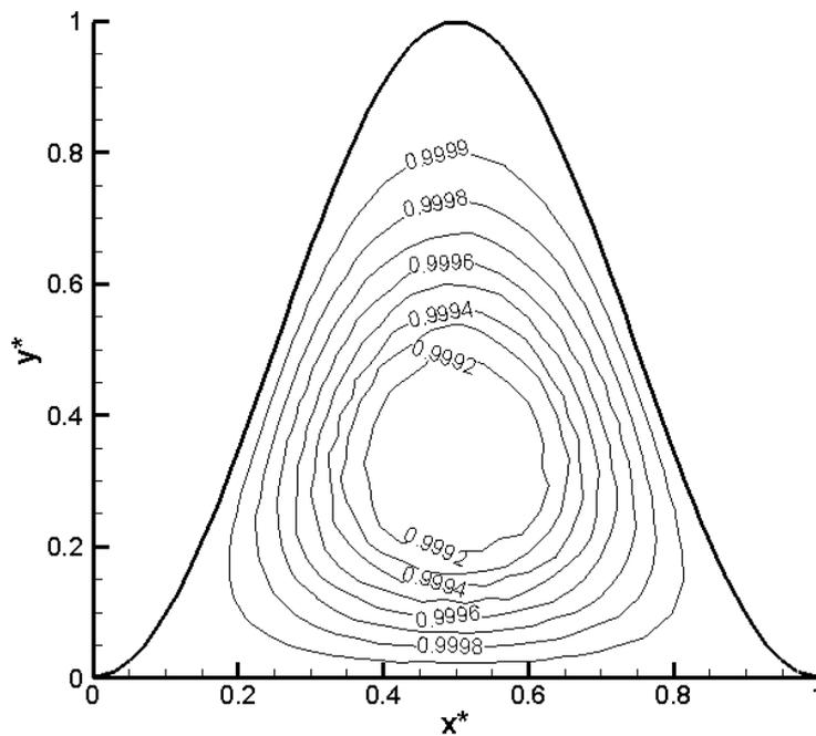
Fig. 4. dimensionless temperature contours on duct cross section,  $a/b=1.0$
