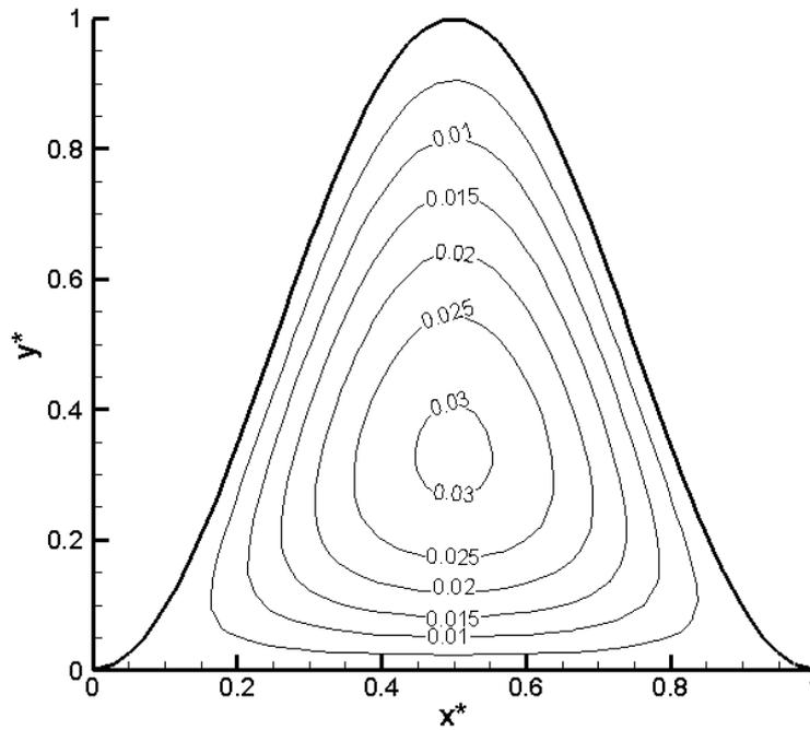
Fig. 3. dimensionless velocity profiles  $u^*$  on duct cross section,  $a/b=1.0$
