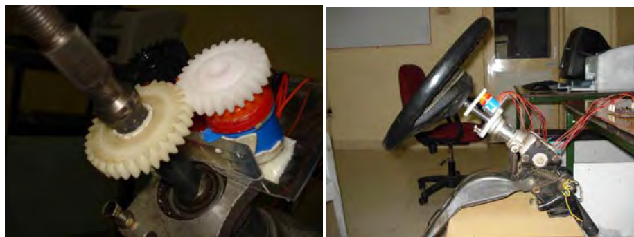
Fig 4 Implementation of sensor system in car steering
