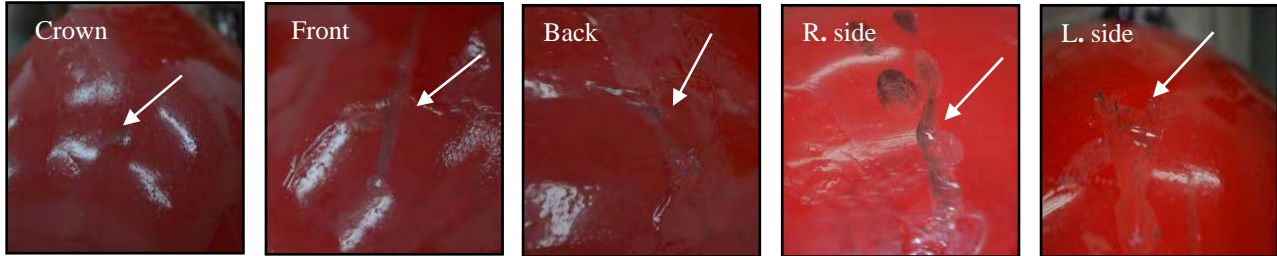
Fig.13. The impact damages occurred on the 100% polyester helmet composite shell on different impact sites.
