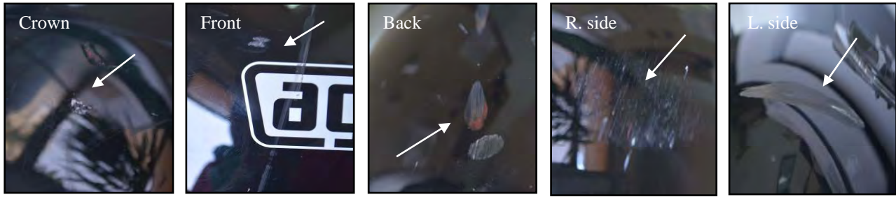
Fig.22. The damages occurred on the ABS helmet at different impact sites.
