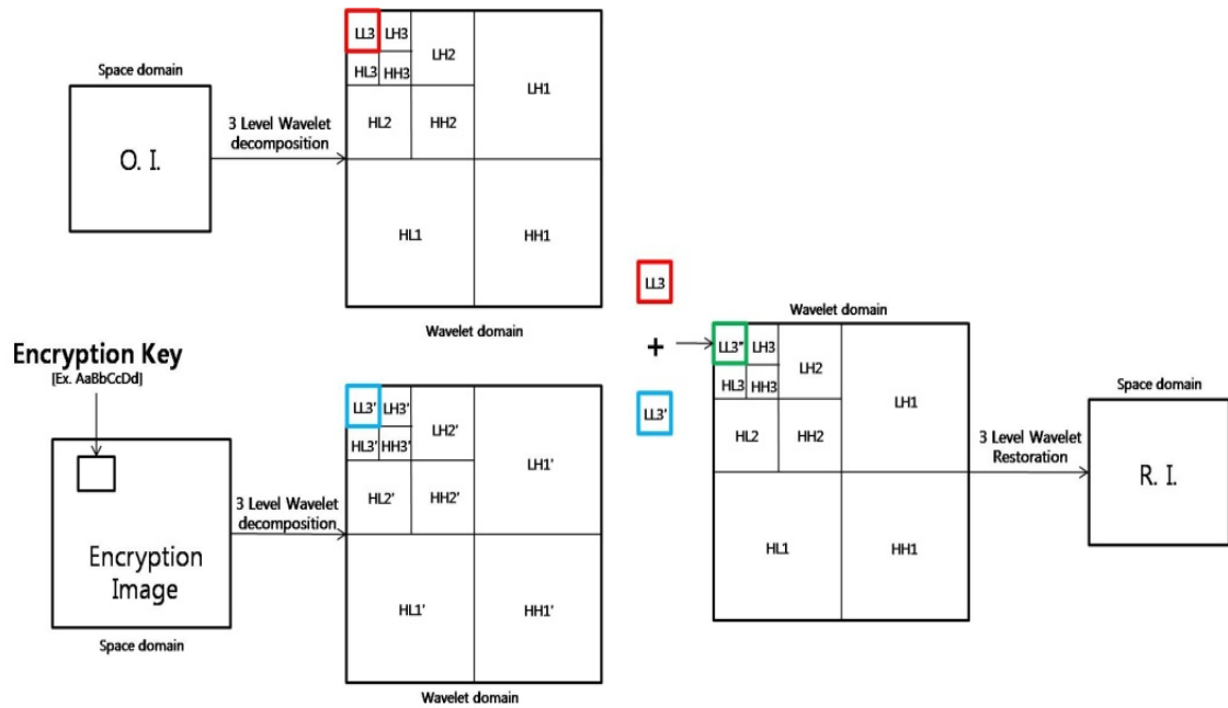
Fig. 3. Proposed wavelet watermarking embedded scheme (O.I and R.I mean original and resulting images.)
