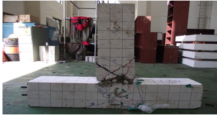
Fig.8. Fracture shape, TCJ-1
