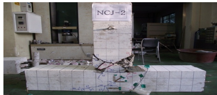
Fig.10. Fracture shape, NCJ-2
