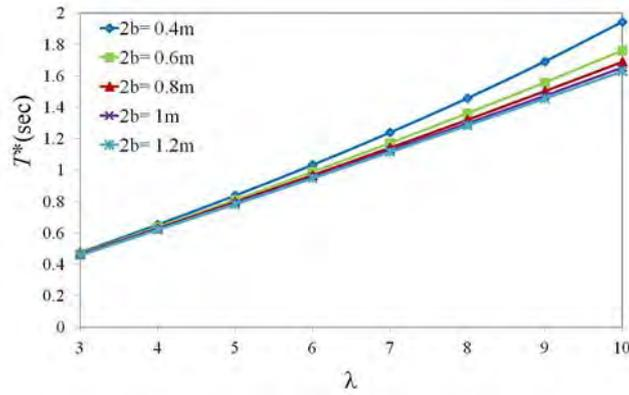
Fig. 3. Relation between the slenderness  $\lambda$  and the stabilized period  $T^*$ , for  $I = 0.15$ ,  $C = 0.6$  and different values of  $b$
