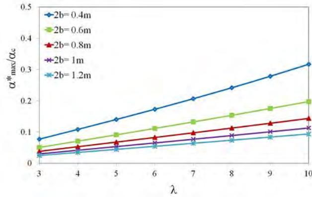
Fig. 6. Resonance spectra in terms of the ratio  $\alpha^*_{\max}/\alpha_c$ , for  $C = 0.6$  and different sizes of the base
