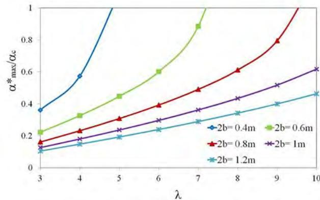
Fig. 8. Resonance spectra in terms of the ratio  $\alpha^*_{\max}/\alpha_c$ , for  $C = 0.8$  and different sizes of the base
