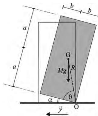
Fig. 1. Rigid rocking block system
