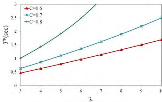
Fig. 5. Relation between the slenderness  $\lambda$  and the stabilized period  $T^*$ , for  $2b = 0.8 \text{ m}$  and different values of  $C$
