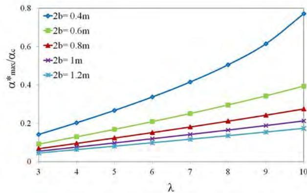
Fig. 7. Resonance spectra in terms of the ratio  $\alpha^*_{\max}/\alpha_c$ , for  $C = 0.7$  and different sizes of the base
