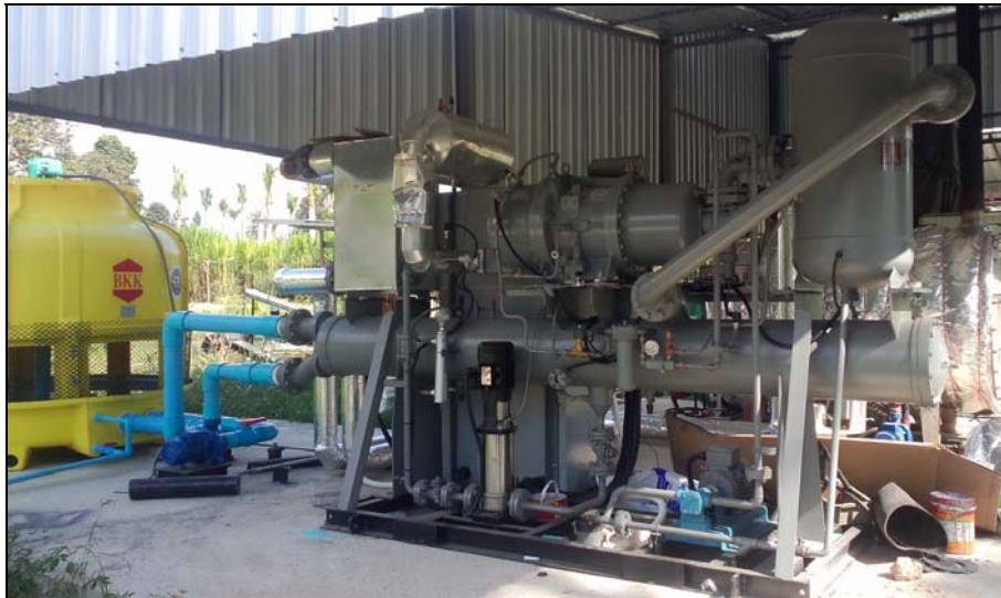
Fig. 2. The ORC Prototype with using R-245fa as working fluid.
