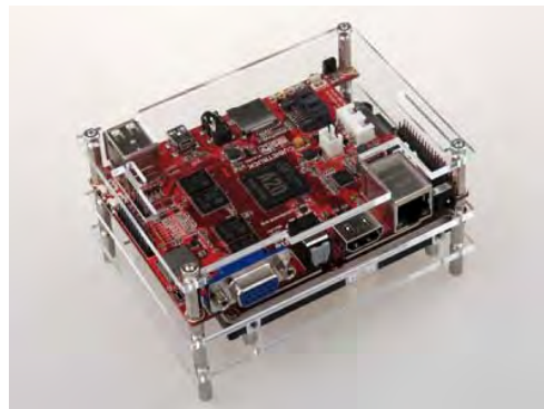
Fig. 8. Single Board Computer – Cubietruck
