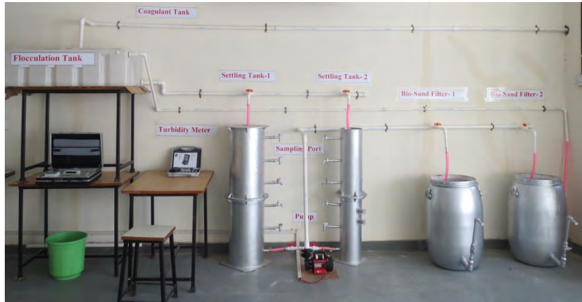
Figure 1 Schematic sketch of Pilot treatment plant
