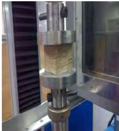
Fig. 4. Composite is vertically positioned before quasi-static compression loading.
