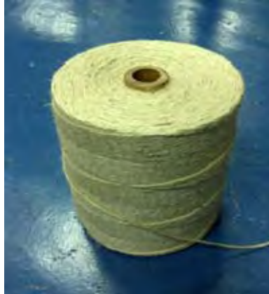
Fig. 1. A bundle of an as-received kenaf yarn fiber.
