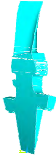
Fig. (5). Computational model for turbocharger TK-32 turbine rotor wheel's strength analysis.
