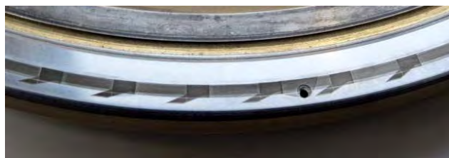
Fig. (18). A sleeve piece with hydrodynamic grooves after testing
