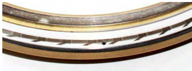
Fig. (15). A sleeve piece with hydrodynamic grooves
