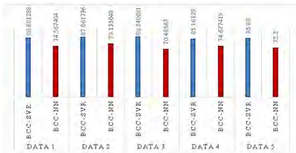
Figure 5 Comparison BCC-SVR with BCC-NN based on EDP for experimental data sets (2-Fold) for error percentage less than 5%
