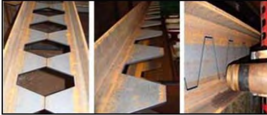
Fig.1. Zigzag Flame Cutting – Castellated Beam
