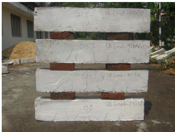
Fig. 15. Failure mode of M60 Beams- 7th day
