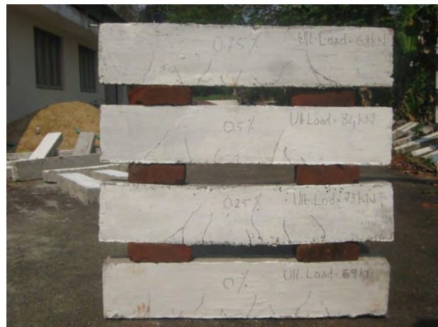
Fig. 12. Failure mode of M40 Beams- 7th day
