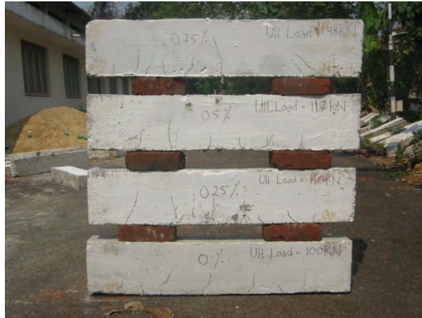
Fig. 16. Failure mode of M60 Beams- 28th day
