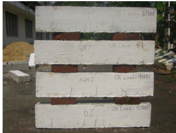
Fig. 13. Failure mode of M40 Beams- 28th day
