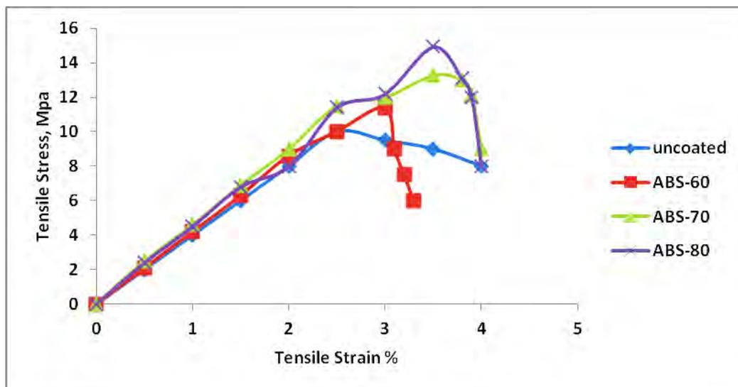
Fig. 6. Tensile Stress vs Tensile Strain for Coated and Uncoated FDM-ABS Samples
