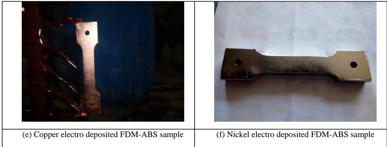
Fig. 3. Electroplating of FDM – ABS Tensile Samples.
