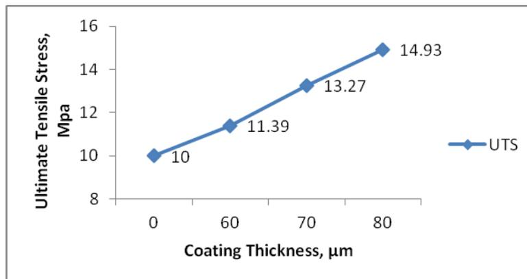
Fig. 4. UTS vs Coating Thickness for FDM-ABS Electroplated Samples
