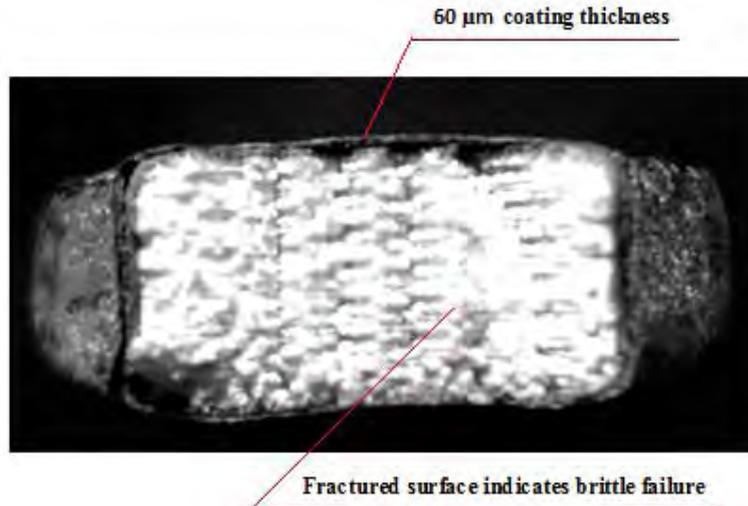
Fig. 5. Enlarged View of Fractured Surface of Tensile Sample.
