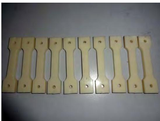
Fig. 2. Developed FDM-ABS Tensile Samples
