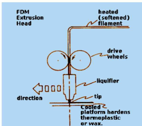
Fig. 1. Fused Deposition Modeling [9]
