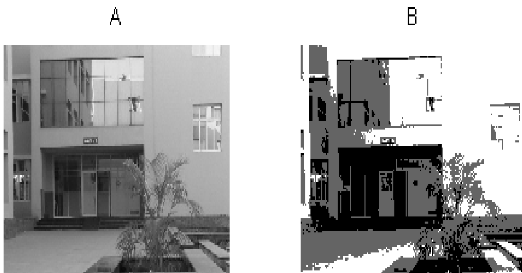
Fig.4. Multilevel thresholding of kiit.jpg(256×256) using proposed PSO ; (A) Original Image (B) Segmented Image
