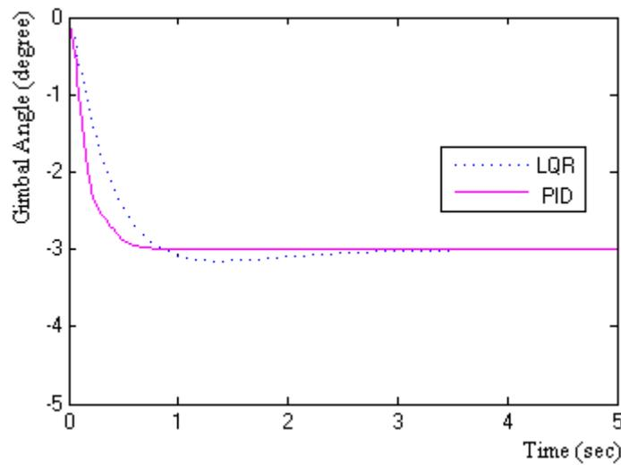
Fig. 9. Response for Deflection of  $-3^{\circ}$
