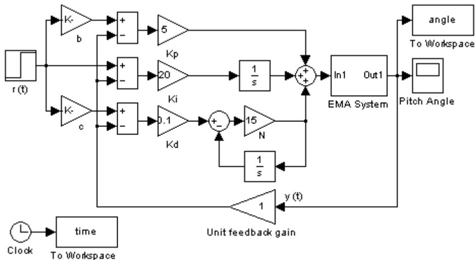
Fig. 6. Gimbal angle control by SW-PID Controller
