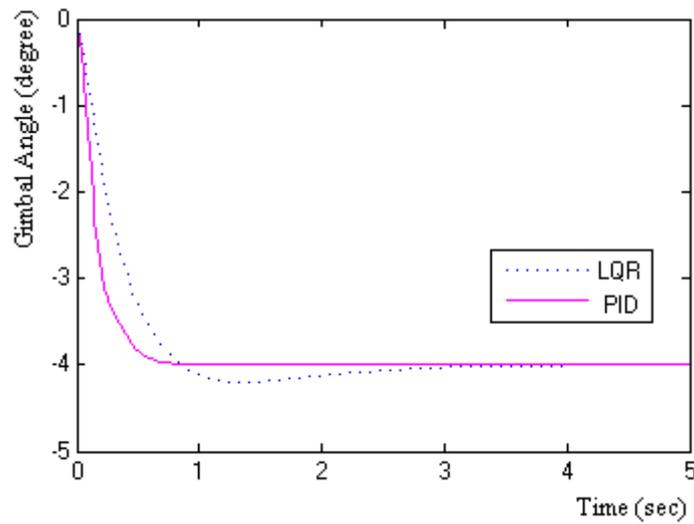
Fig. 8. Response for Deflection of  $-4^{\circ}$
