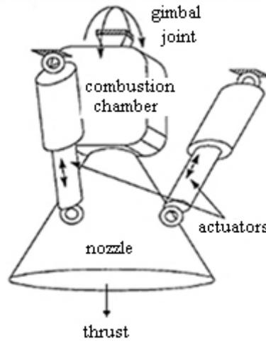
Fig. 2. Nozzle and Actuator placement
