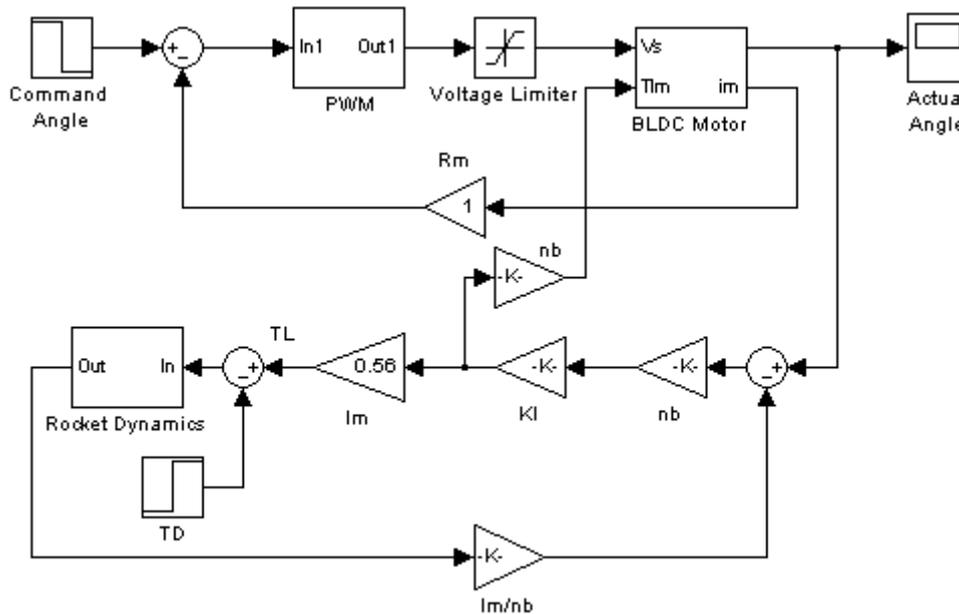
Fig. 3. Open Loop Electro Mechanical Actuator System
