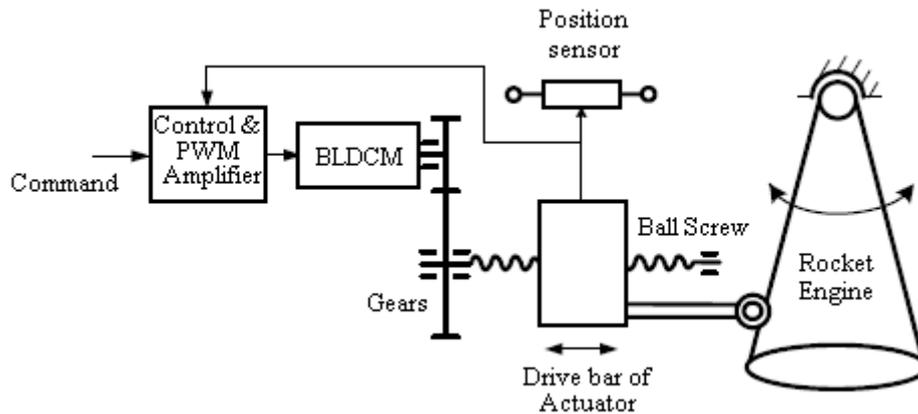
Fig. 1. Electro Mechanical Engine Gimbal Control System
