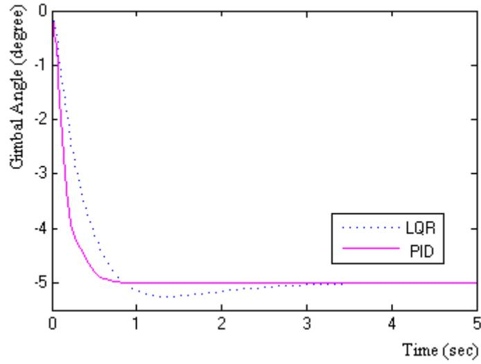
Fig. 7. Response for Deflection of  $-5^{\circ}$
