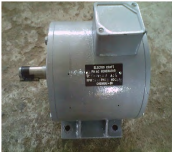
d) PMAC Generator
