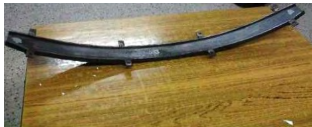
Fig 1. Die used for composite leaf spring fabrication
