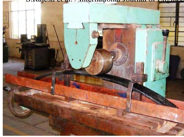
Fig. 4. Cam arrangement set up for cyclic loading in milling machine
