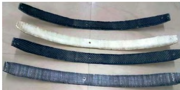
Fig 2. Fabricated composite leaf spring.
