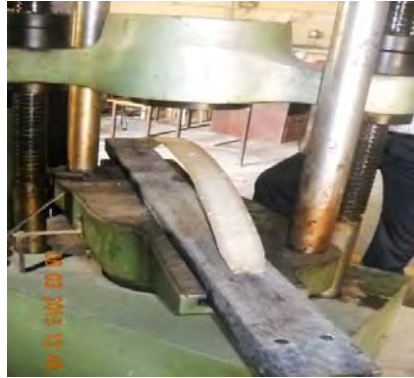
Fig. 3. Testing of composite leaf spring using Universal Testing Machine
