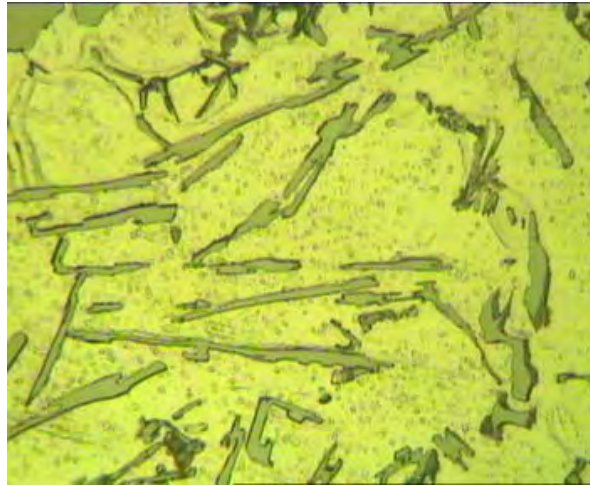
Fig. 21. Microstructure of Aluminium Specimen under 500 X Magnification at another location
