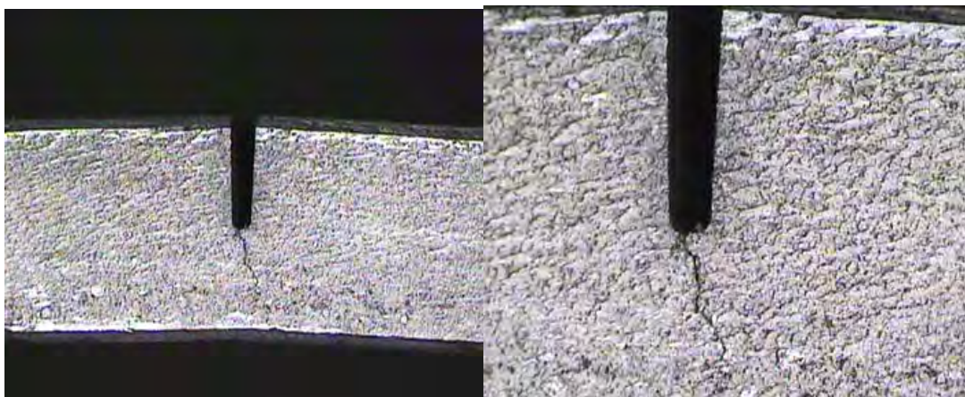
Fig. 18. Crack Growth Path in the Aluminium-Silicon Carbide Specimen with a/d Ratio of 0.5 under 10 X Magnification and 20 X Magnification
