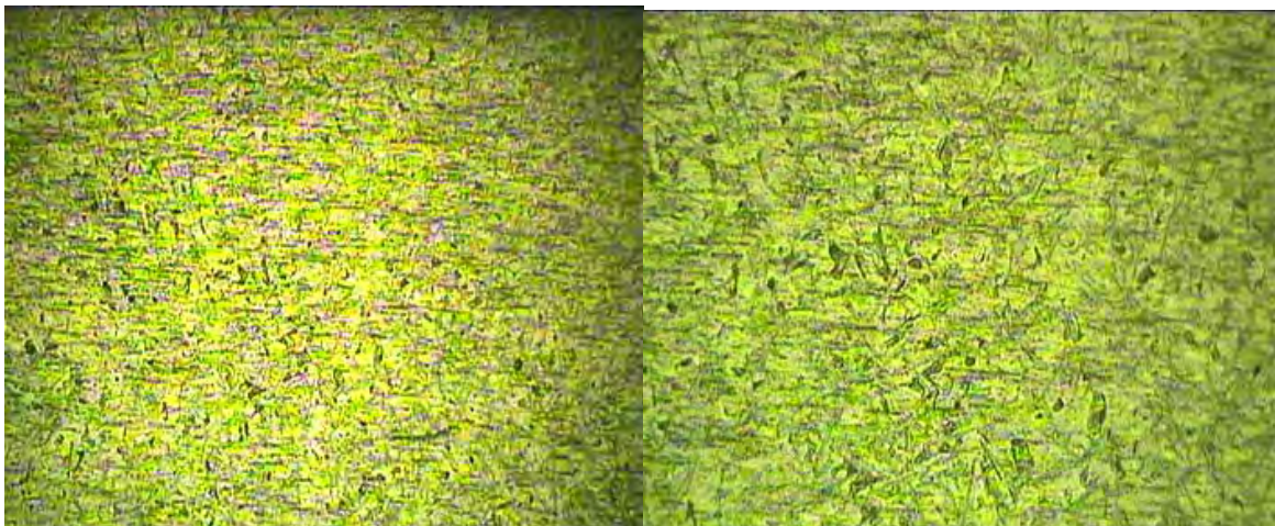
Fig. 22. Microstructure of Aluminium-Silicon Carbide Specimen under 50 X Magnification and 100 X Magnification
