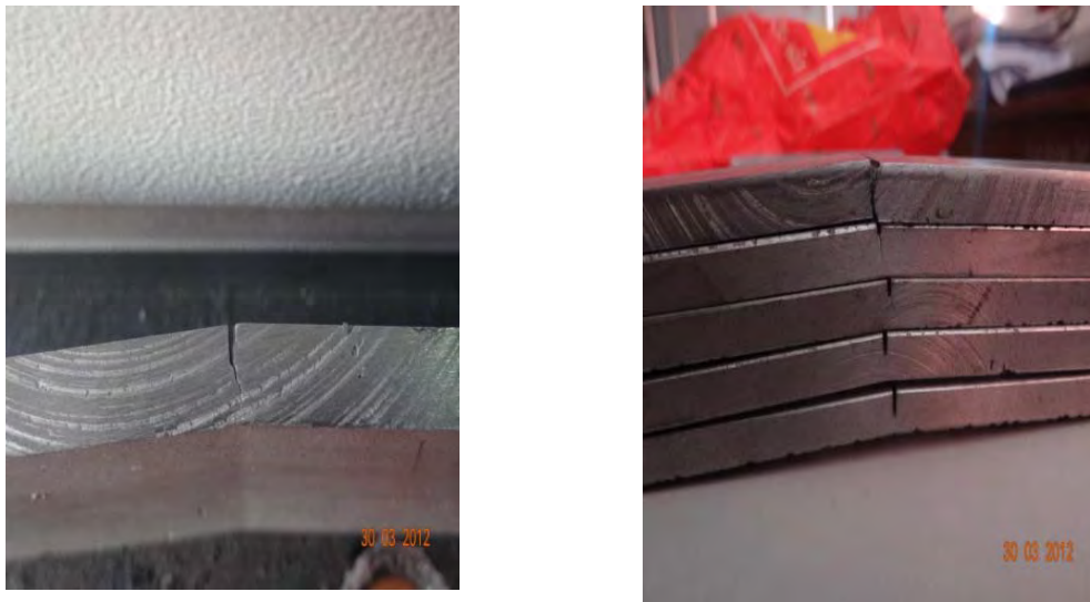
Fig. 3. An Aluminium Specimen with crack and Multiple Al-SiC Specimens with cracks in the depth direction
