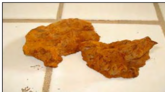
Fig. 9 – Rust deposit from a forsaken pipe
