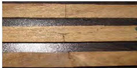
Fig. 5. Failed specimens of teakwood beam without finger joint - edgewise test
