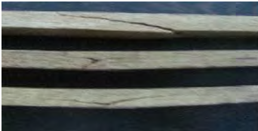
Fig. 7. Failed specimens of teakwood beam without finger joint- flat wise test
