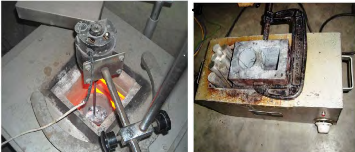
Fig. 2 Stir casting equipment (a) Electrical furnace (b) Preheated permanent mould
