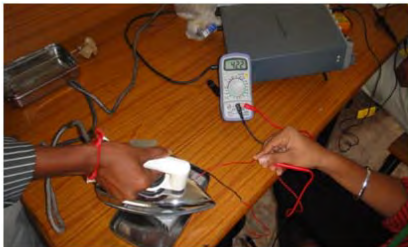
Fig.16. Testing of Thermoelectric Generator (TEG)
