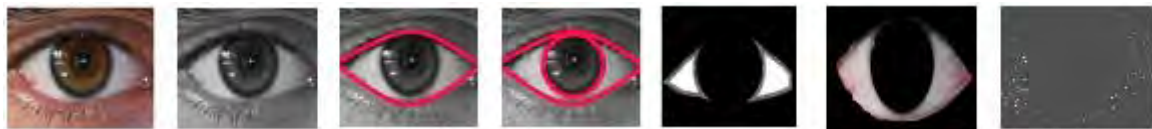
Fig. 4. (a) Input eye image (b) Grayscale image (c) Eyelid detection (d) Iris boundary detection (e) Sclera mask (f) Segmented Sclera (g) Vessel pattern- after morphological operation
