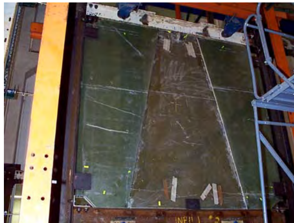
Fig. 2. Geometric Configuration of the PMC Infill Wall [1]
