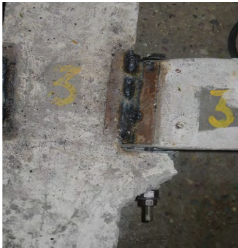
Fig. 5. Connections of Beam-column joint using Steel bolts and L-angles
