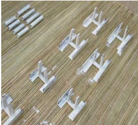
Fig. 4. Steel bolts and L-angles used for connection of joints
