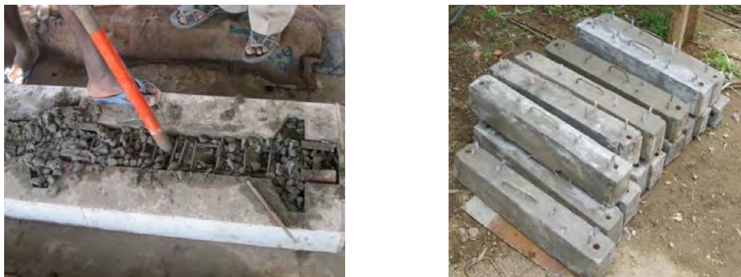
Fig. 3(b). Concreting of precast column and completed beam specimens
