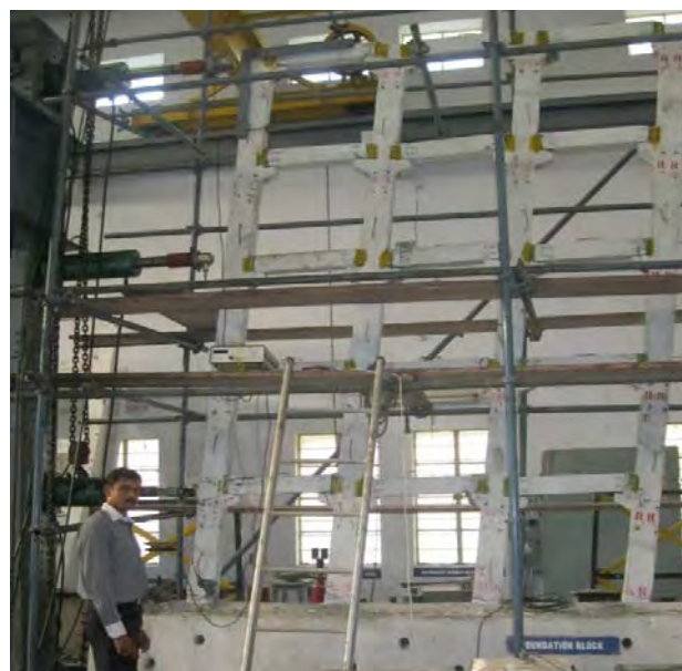
Fig. 8. Precast model frame after testing
