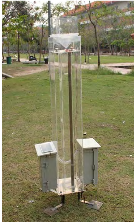
Fig. 6: The prototype of the proposed rainfall telemetry system
